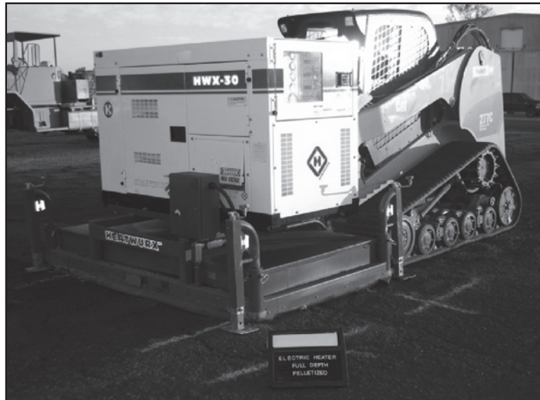
Figure 36. Electric heater being placed on repair area.
