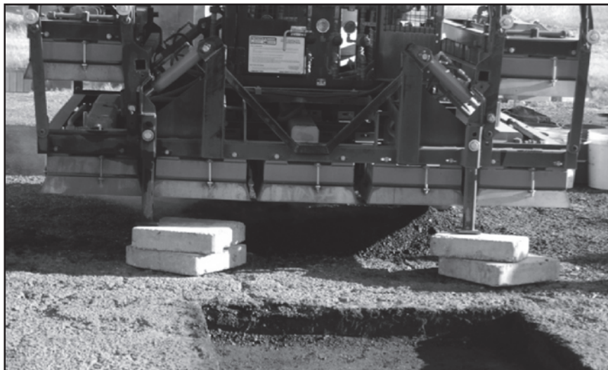
Figure 47. Propane heater keeping rejuvenated stockpile hot.
