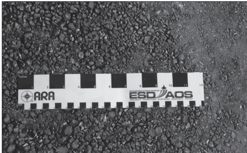
Figure 58. Post-compaction repair surface (PD-2).
