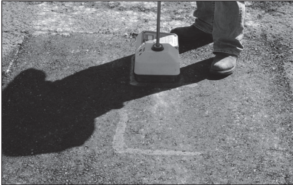
Figure 53. Nuclear density gauge taking measurement.
