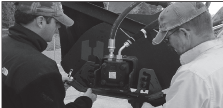
Figure A4. Manually adjusting processor cut depth.
