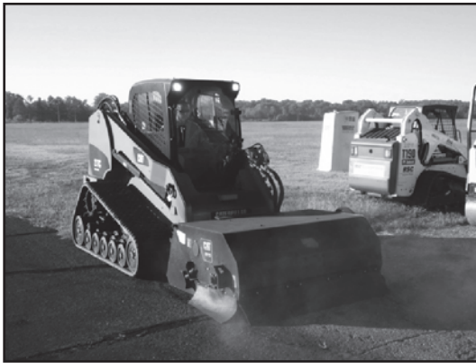
Figure 33. Skid steer mounted broom attachment.
