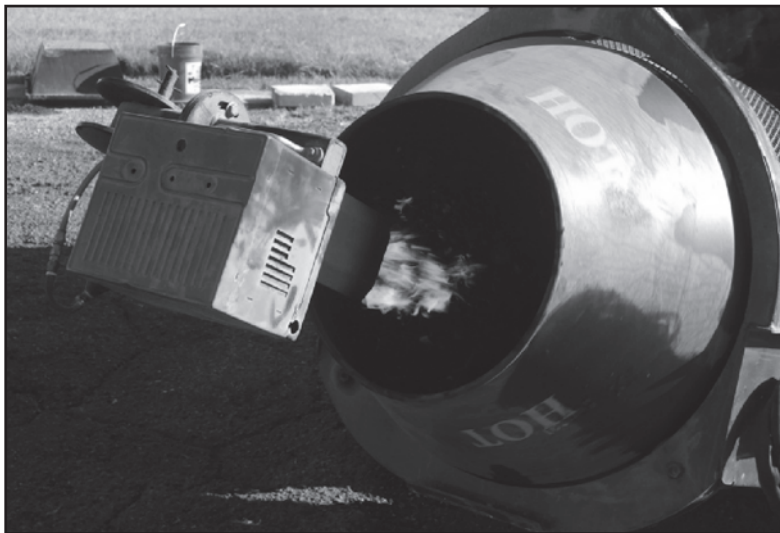
Figure A7. Additional heat being applied to rap material.
