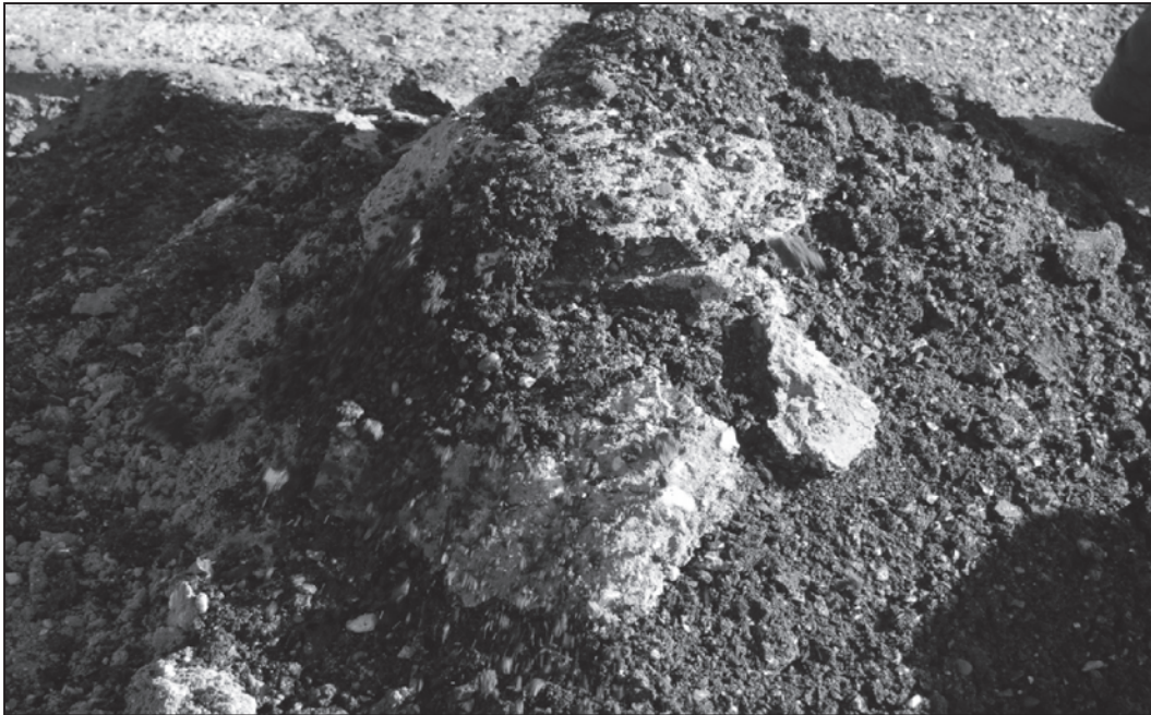
Figure 57. Disturbed base material mixed with excavated RAP.
