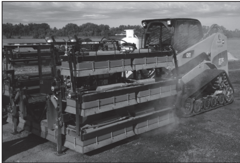
Figure 37. Propane heater during initial heat sequence.
