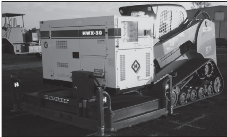
Figure A2. Heater being placed over repair area.
