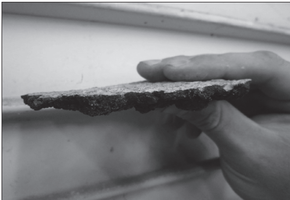
Figure 81. Asphalt material from oxidation test.
