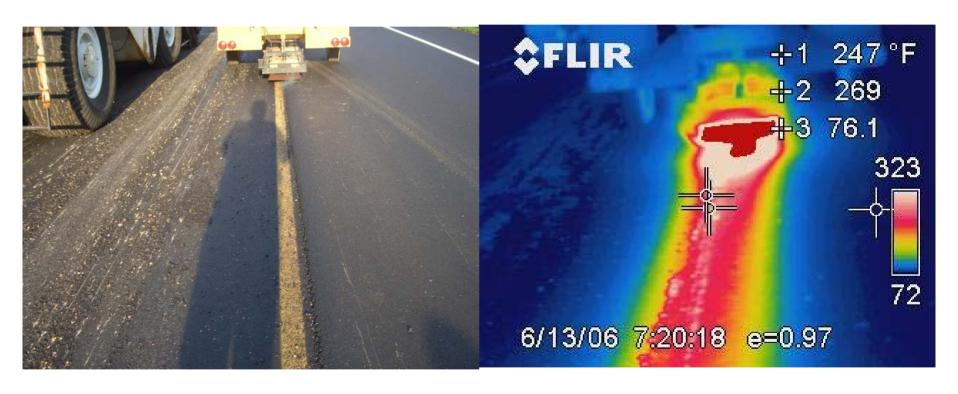
The only "smoke" is steam being driven off the surface, no evidence of blue smoke or light ends of the bitumen were noted.
