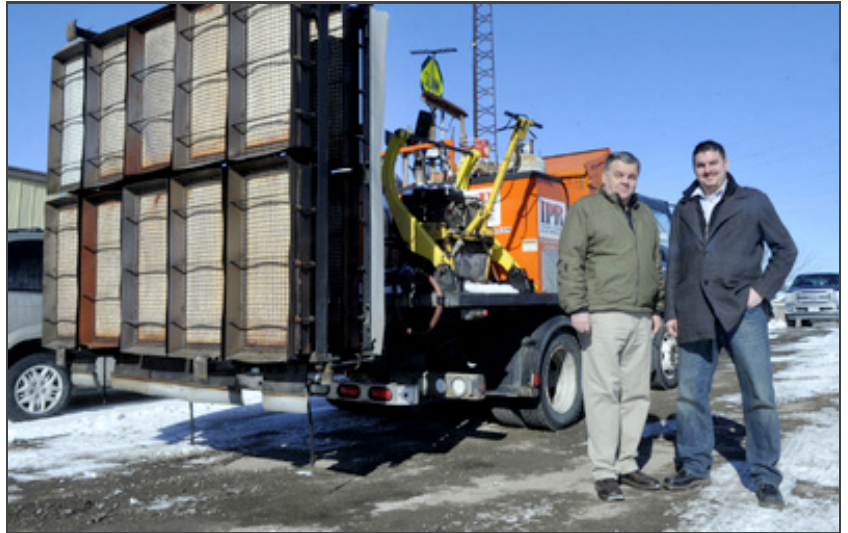
rec-heat design-13. Bob Kieswetter (left) owner of Heat Design Equipment Inc., and his son, Matt, stand next to an infrared asphalt heater used to repair potholes and road cracks. Record staff Source: Record staff
